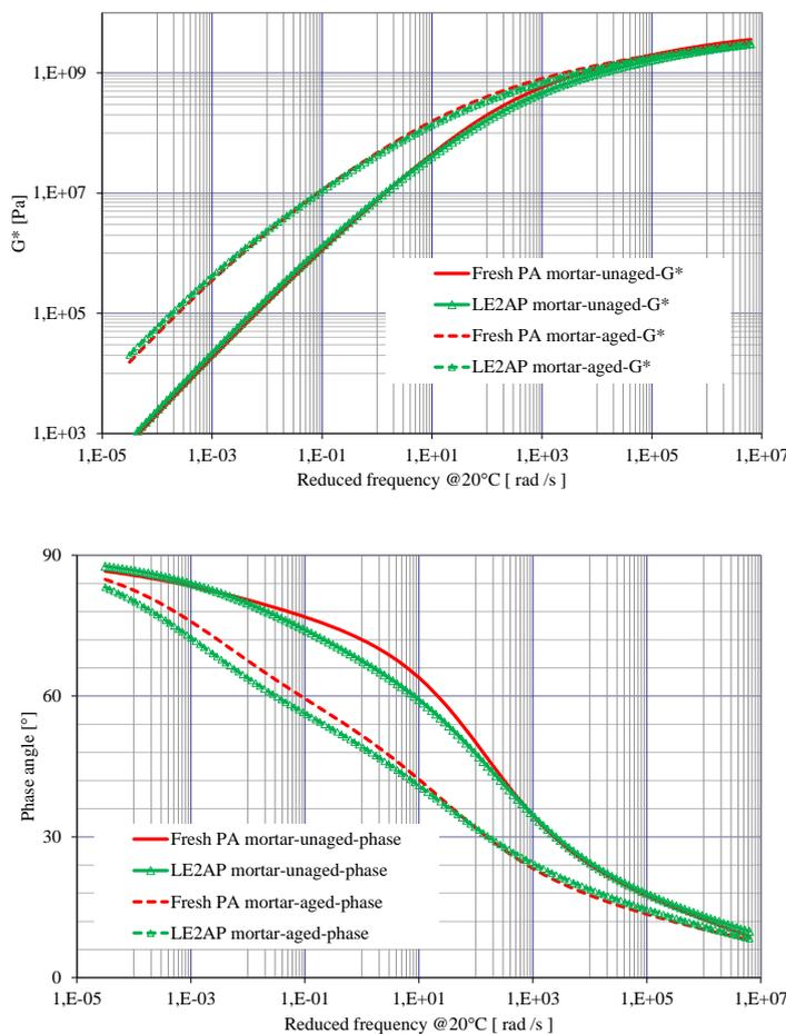
Figure 5. Response test on mortar columns
