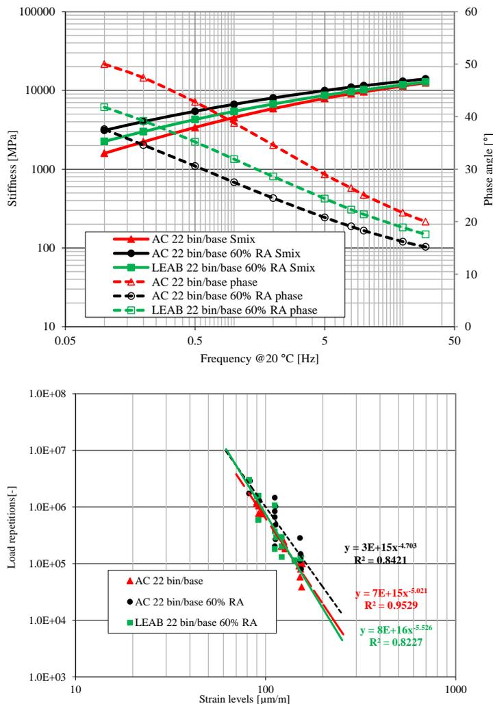
Figure 3 Results of stiffness and fatigue tests
