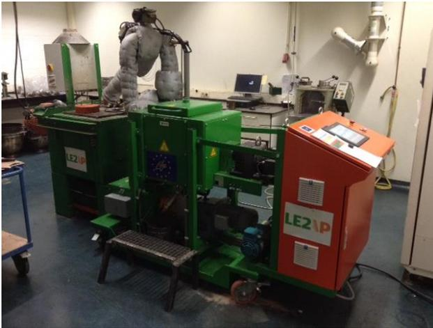
Figure 6. Illustration of mortar foaming device
