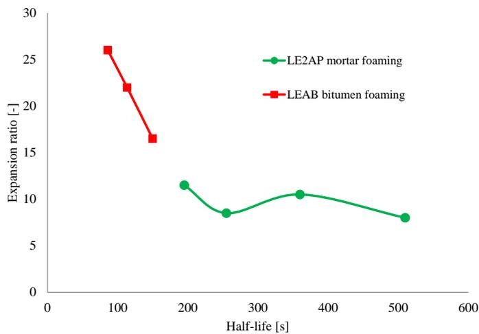
Figure 7. Results of the mortar foaming tests
