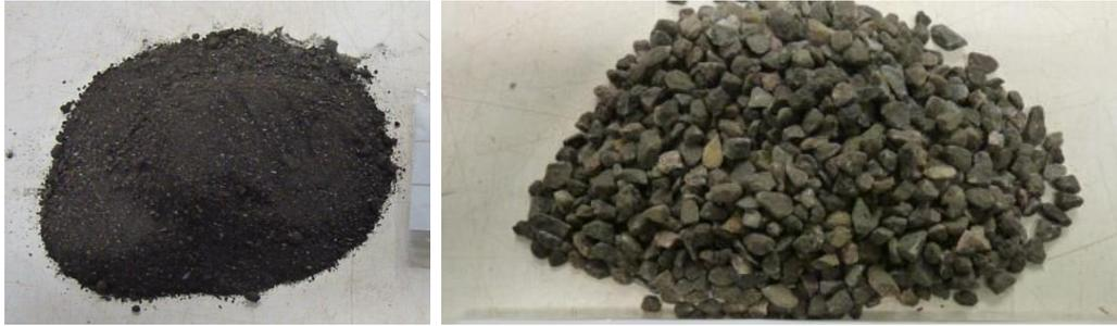
Figure 4. Materials obtained after decomposition: reclaimed mortar sand and PA-stone
