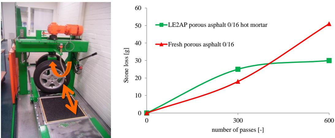
Figure 8. Illustration of the ARTE and results of the ARTE tests
