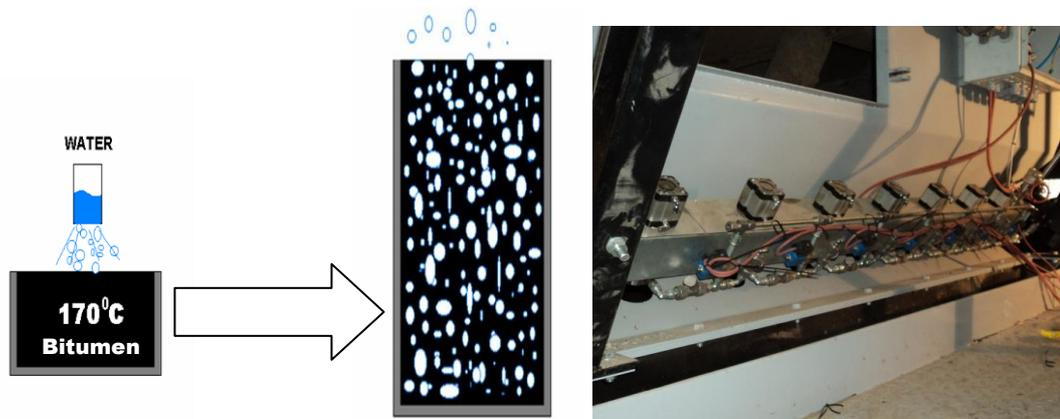
Figure 1 Principle of bitumen foaming and LEAB foaming installations in the asphalt plant (Jacobs et al 2010)
