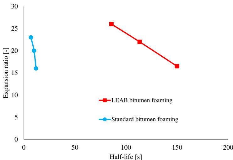
Figure 2 Results of foaming properties of LEAB bitumen
